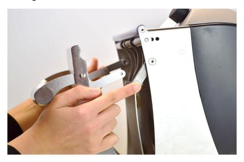
Note: it is possible to disengage first the rods and then the black locking parts.
