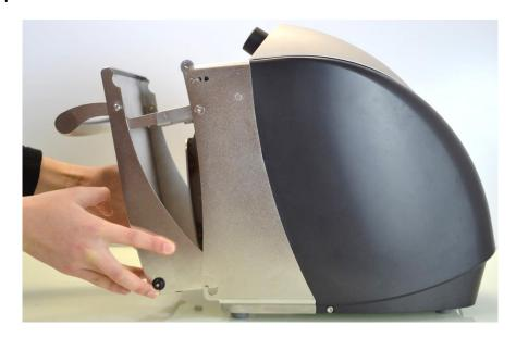
Successively disengage the joints from the articulated rods holding the door.
