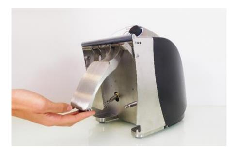
• Press the central spring (1), holding together the 2 paddles as explained below, to disengage the upward fixations (2) from their holes:
