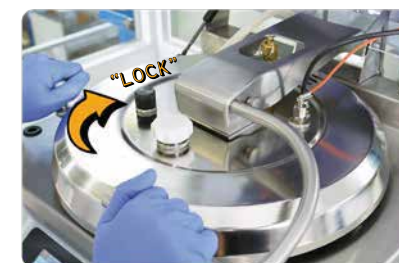
Safety lock with 12 hooks !
